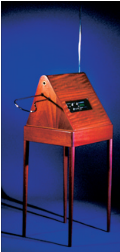
FIG. 8: The Big Briar Ethervox theremin is a world-class performance instrument with extensive MIDI capabilities.
