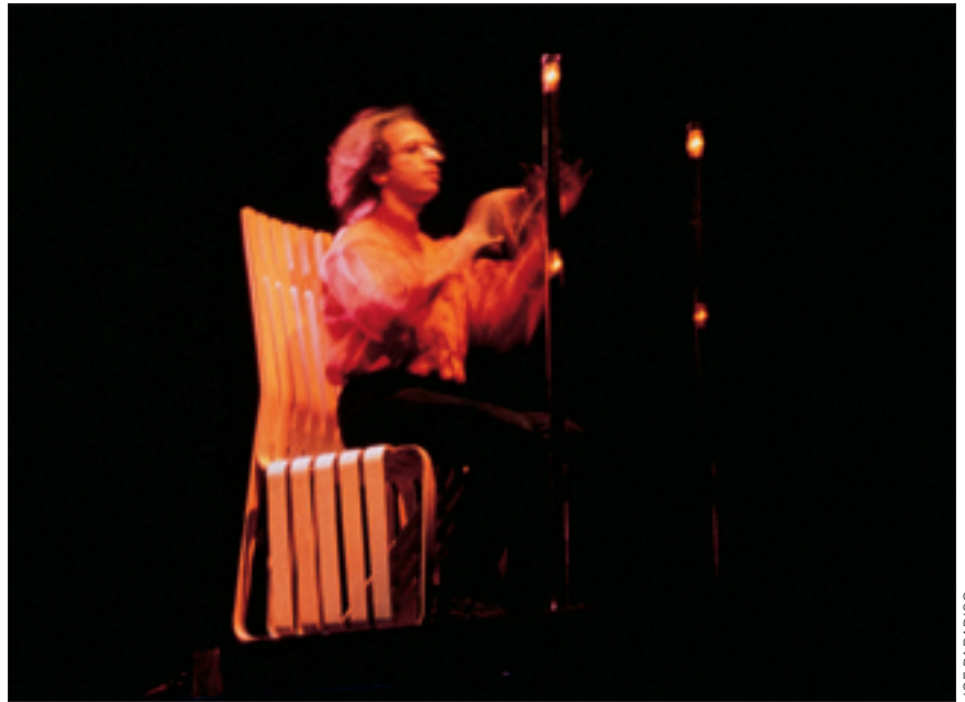
FIG. 11: Tod Machover of MIT's MediaLab performs in the Sensor Chair, which senses the position and movement of the performer's arms and upper body.
