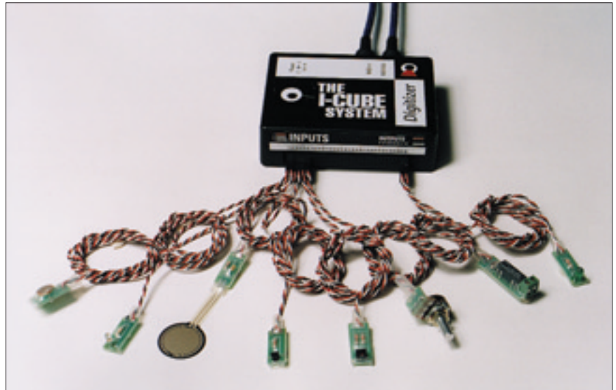
FIG. 7: All of the I-CubeX sensors come prewired and ready to use—no soldering is necessary. As many as 32 sensors can be used with the system at one time.
