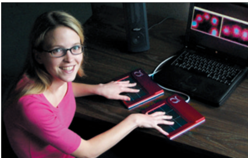
FIG. 1: The MTC Express, from Tactex Controls, can track the Velocity and position of several stimuli simultaneously.
